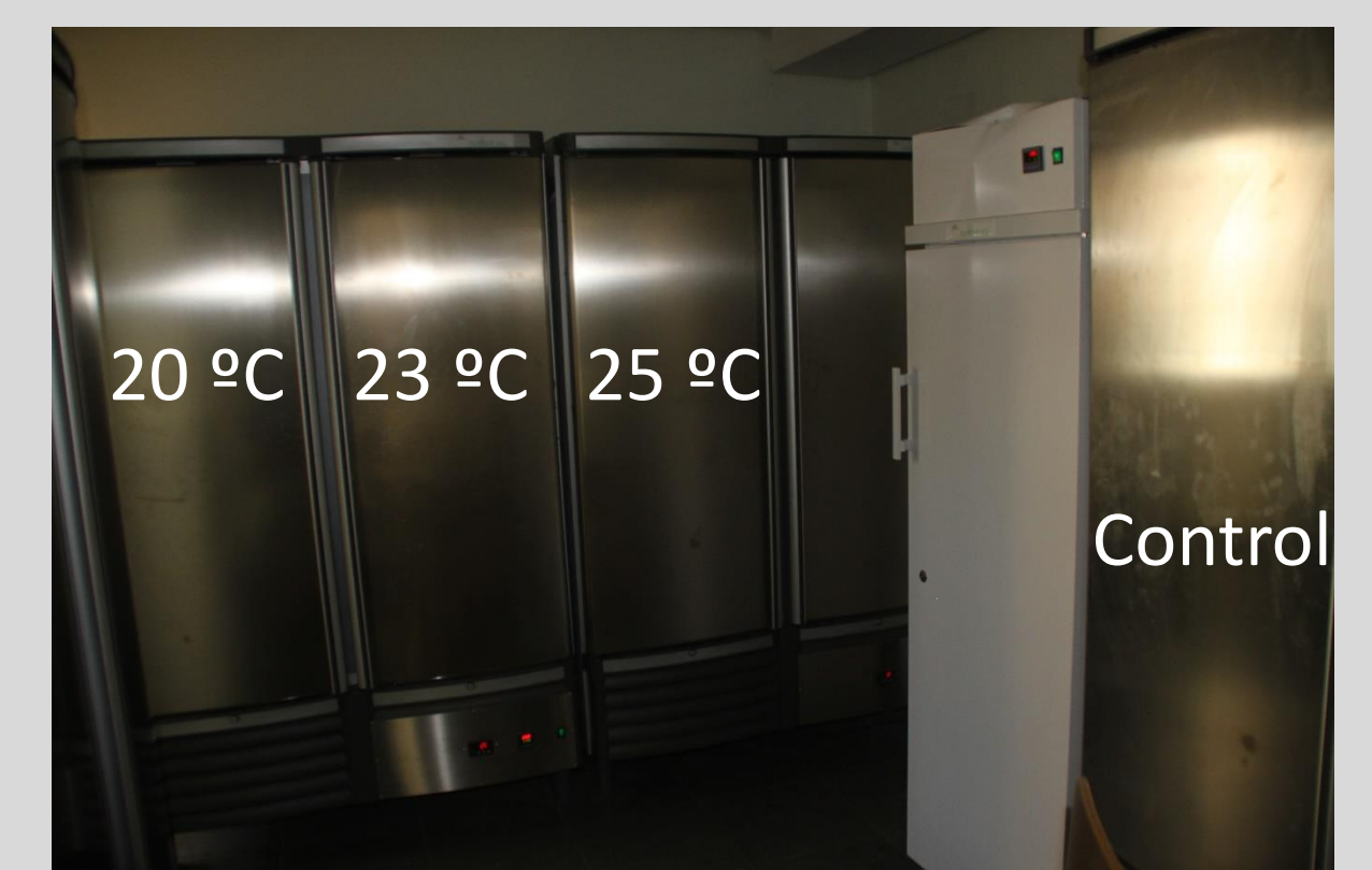
Climatic chambers at the ICAM (UCLM, Toledo) used to carry out long-term experiments
