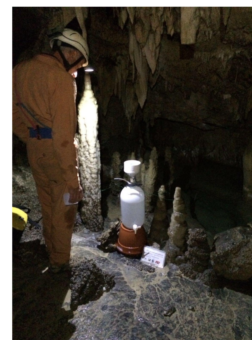
Fig. 5. Sampling device for collecting the ceiling drip and retain animals.
